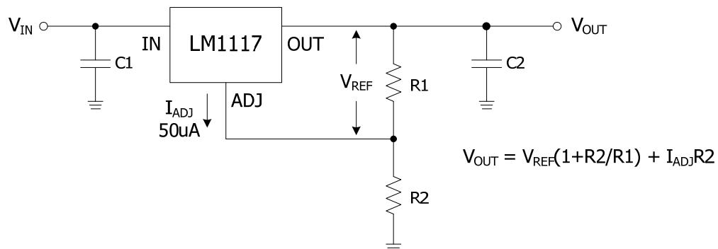
Fig.2 Typical Adjustable Regulator
