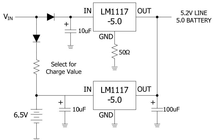
Fig.6 Battery Backed-up Regulated Supply
