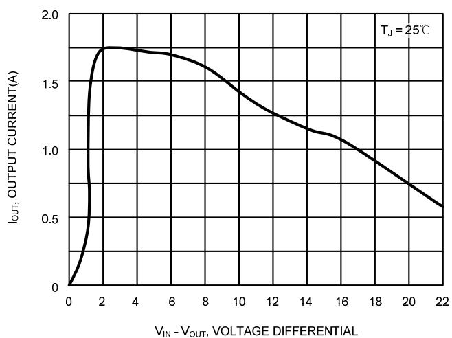
Fig.9 OUTPUT SHORT CIRCUIT CURRENT VS DIFFERENTIAL VOLTAGE
